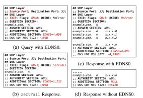
Figure 6. DNS Query and Response Packet Examples. Red-signated Fields will be Assigned Different Values Based on the Scenario.
