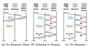
Figure 4. DNS Resolution under the DNS Timeout Mechanism.
