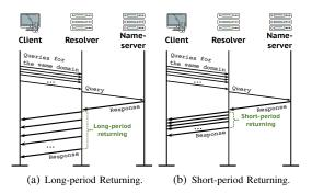
Figure 7. DNS Response Returning Examples of Resolvers.
